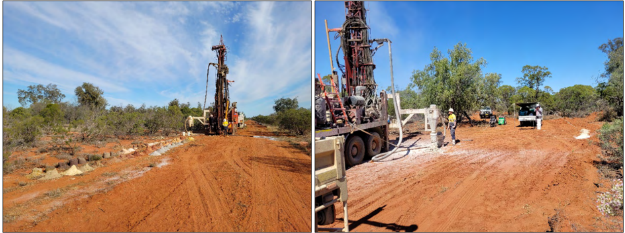
Figure 8: Left) Typical set up of the aircore rig drilling a vertical hole, with samples in the foreground as 1m piles. Right) aircore rig with white cyclone used to collect sample; field ute in background used as platform for geological logging.
